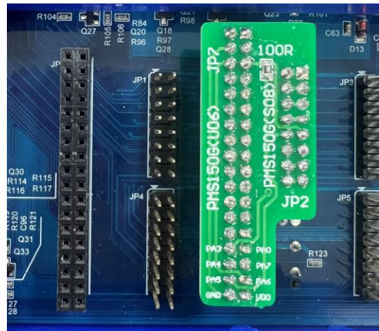
Fig. 15: JP2 Physical connection diagram
